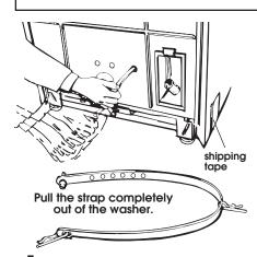
Remove tape that covers shipping strap. Pull to completely remove the shipping strap with 2 cotterpins from the inside of the washer.
